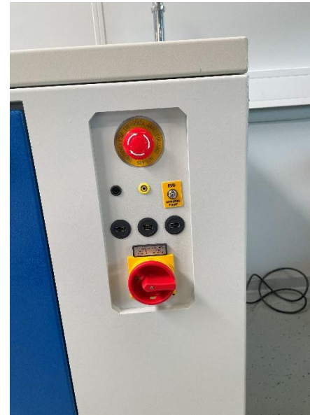
Right Main switch, Emergency stop, USB ...
