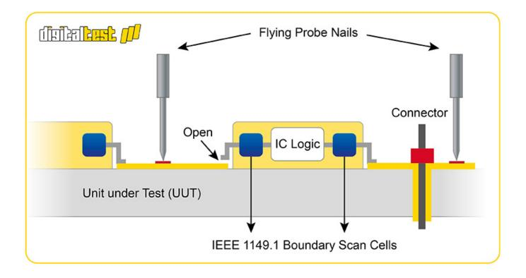
With the boundary scan upgrade to our Flying Probe the needles can act as virtual JTAT/Boundary Scan cells. This increases fault coverage, since now the conductor paths that otherwise could not be reached can also be tested.
