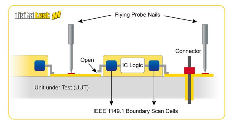
With the boundary scan upgrade to our Flying Probe the needles can act as virtual JTAT/Boundary Scan cells. This increases fault coverage, since now the conductor paths that otherwise could not be reached can also be tested.
